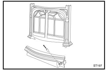
Fig. 27 Attach the handle to the control door.
